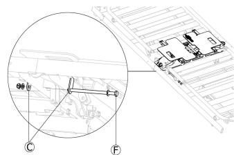
Fix the main module onto the crossbars of the mattress support frame, by placing the carrige-bolt  $^{\textcircled{e}}$ , trough the designated bracket on the main module  $^{\textcircled{e}}$ , washer and nut, from underneath on both sides of the bed.
