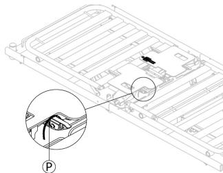
Cut all the zip ties ® to release the wings, and fix the main module flat with the crossbars of the mattress support. Make sure new zip ties are placed in the same location when the main module is to be removed from the bed.
