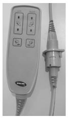
Connect the hand control to cable  $\circledR$  and connect the power cable ข to the mains. The hand control cable is marked v on the cable clip corresponding to v on the control box cable.
