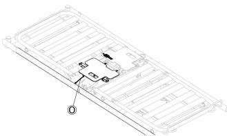
Ensure that the main module is placed in the middle of the mattress support frame and the distance 0, to the side tubes is the same on both sides.
