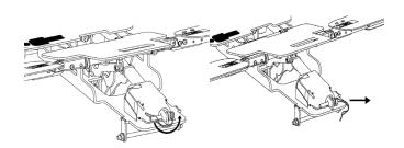
After the pin is removed, lift the motor out of the support and slowly lower the wing.
