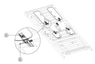
Connect the four arms with the main module, following the representation on the arms label shown in the zoomed image 0, the black shaded area on the sticker represents the location were the arm must be placed. Fix the four arms with the Allen bolts from set 6 and tighten the lock nuts facing inwards. Ensure the safety washers are placed on the lock nut side.
