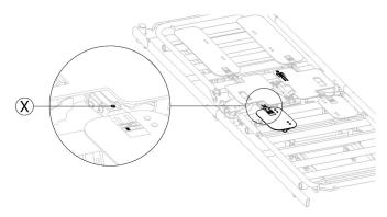
To adjust the position of the arms adjust the bolt  ${\mathfrak B}$  until the arms are in a horizontal position.
