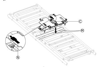
Place the main module © onto the crossbars M, following
