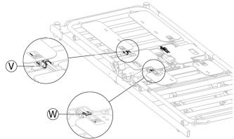
Ensure that the head arms are mounted on the telescopic bracket
