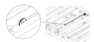
Unscrew and remove the distance stick, located at the cross bar of the mattress support head section, and keep it available for remounting, when the Soft Tilt is removed again from the bed.
