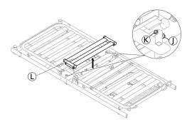
On each side of the bed, remove the nut 1 and bolt 6 using two 13 mm keys to remove the slats assembly 1 from the bed, and keep it available for remounting, when the Soft Tilt is removed again from the bed.
