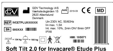
The product label is placed on the main module of the Soft Tilt and contains the main product information, including technical data.
