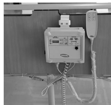
Collect the motor cables in a bundle and tighten it with a zip tie, move the bed up and down to make sure that the bundle is not clinging on any bed parts and moves freely.
