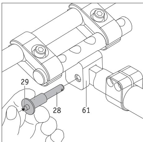
In order to operate the wheelchair with the e-pilot again after transport, you have to re-attach the cross strut [60] to the wheelchair.
