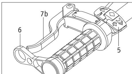
Apart from the two brake levers [7a, 7b], the battery pack must be switched on in order to use the control elements (see chapter 3.4).
