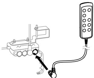
Connect the standard hand control to the empty socket on the junction box.
