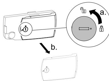
On the control unit turn the lock 90 degrees counter-clockwise to open the lid and remove it.
