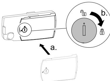
Put the lid back on the control unit and close it by turning the lock 90 degrees clockwise.
