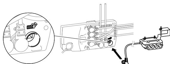
Connect the cable from the junction box to the control unit in the socket labeled with hand control symbol.
