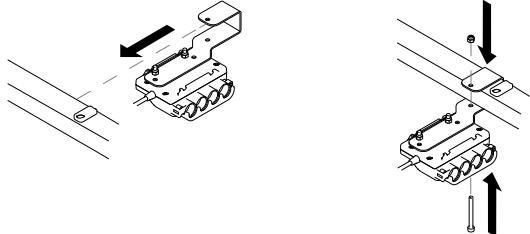
1. Place the mounting bracket of the junction box over the square tube of the mattress support platform.
