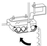
Reinstall the locking cam and ensure it is locked in place.
