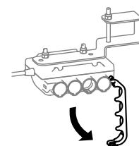
Remove the locking cam on the junction box.
