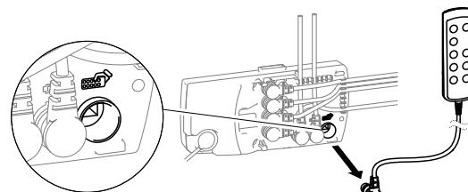
Disconnect the cable of the tethered hand control from the control unit.
