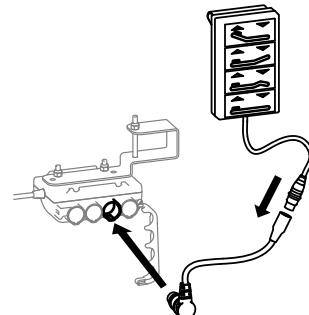
With the adapter cable, connect the rheumatic hand control to the yellow marked socket on the junction box .
