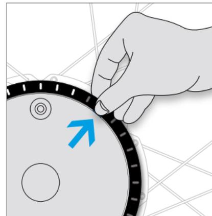
Grip the edge of the ring and press your thumbnail into the notch. Pull outwards at the same time.
