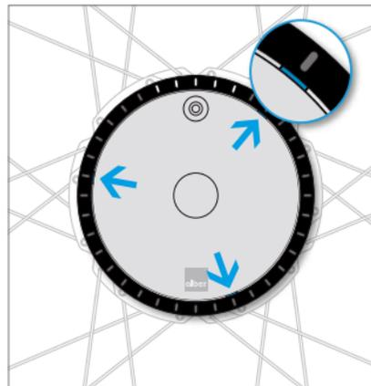
Find one of the three recesses at the outer edge of the cover (between ring and cover).
