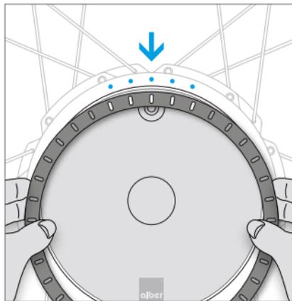
Align the new ring so that the 5 LED recesses correspond to the 5 LEDs on the drive unit.
