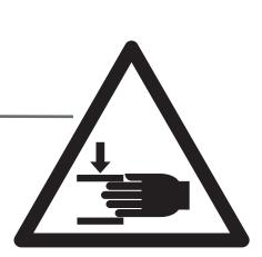
Caution must be exercised when moving or collapsing the anti-tippers, particularly when manually adjusting or activating. As a result of the necessarily high spring force there is a crushing hazard between the holding rod [73] and the clamping piece [72].
