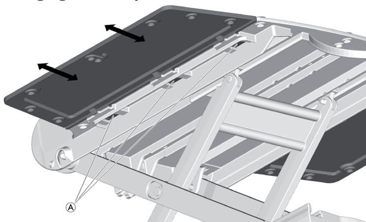
1. Starting from one side press in clips **A** and simultaneously pull out the side flap slowly.
