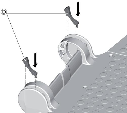
8. Insert the wedge pieces ④ into the seat plate.
