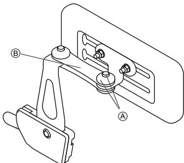
Remove upper screw and friction cap (A).
