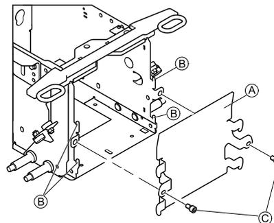
Push the recessed front cover (A) down on the hooks (B).
