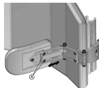
1. Loosen screws (x2) (A) to adjust pad depth.
