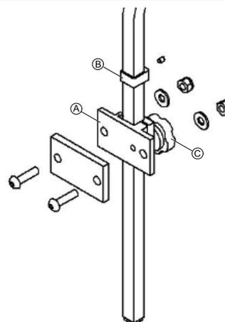
1. Using hardware provided, align and install headrest clamp assembly into existing mounting holes in backrest pan (A).
