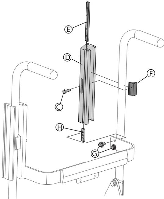
1. Remove hardware **C** securing the back mount **D** to the cane back canes.
