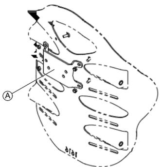
1. Using the hardware provided, align and install the headrest adapter **A** into the existing mounting holes in the back pan.
