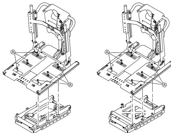
Fig. 7-6 Example of tilt module    Fig. 7-7 Example of anterior tilt wedge
