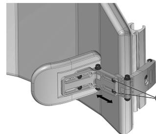
1. Loosen screws (x2) (A) to adjust bracket width.
