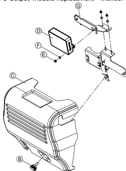
Fig. 15-4 Output Module Replacement—Powered Backrest
