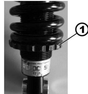
If not, rotate the adjustable spring plate (1) clockwise until the ground clearance is at least 80 mm.
