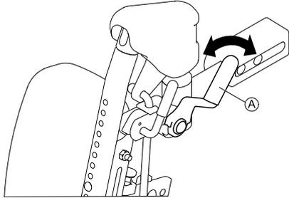
Place lever handle **A** in unlocked position.
