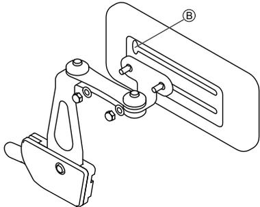
Remove hip pad bracket from mounting slot via cut-out (B).
