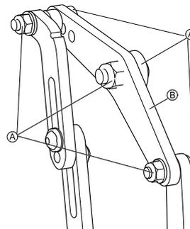
Remove screws, washers and nuts (A).
