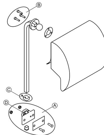
1. Using the hardware provided, align and install the headrest clamp assembly into the existing mounting holes in the back pan **A**.
