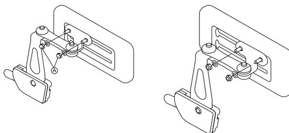
1. Loosen the two screws **A**.
