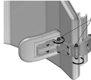
1. Loosen nuts/screws (x2) (A) to adjust pad angle.
