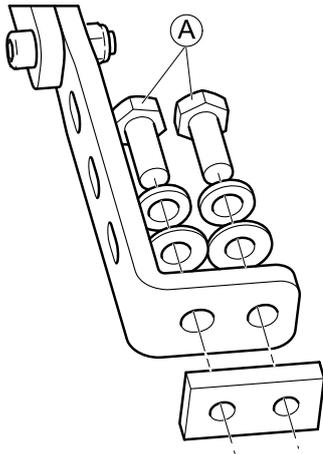
1. Loosen screws **A** on both sides.
