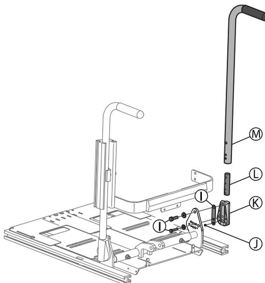
1. Remove hardware (I) securing the back cane (M) to the base.
