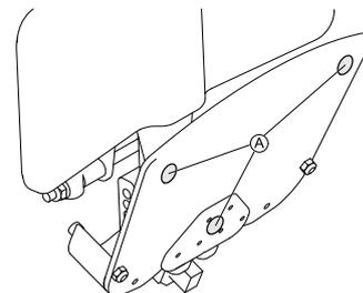
1. Replace worn felt pads **A** on bottom of footboard to avoid damage to the floor.
