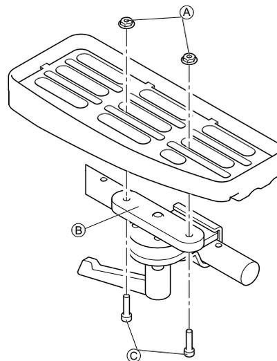
Attach mount plate (B) to armpad body with screws (C) and nuts (A).
