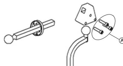
1. Loosen hardware in multi-offset bracket (A).
