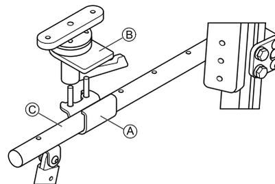
Attach strap plate (A) and clamp plate (B) to armrest tube (C).
