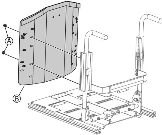
1. Remove hardware **A** securing the seat back **B** to the back canes.
