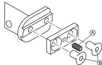
1. Heat grub screw (A) to loosen blocker.
