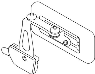
Remove hip pad with bracket, turn upside down and reinstall.
