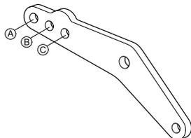
Adjust ESR crankarm to desired shear reduction:
