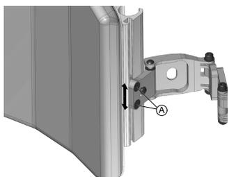
1. Loosen screws (x2) **A** to adjust lateral height (or remove).
