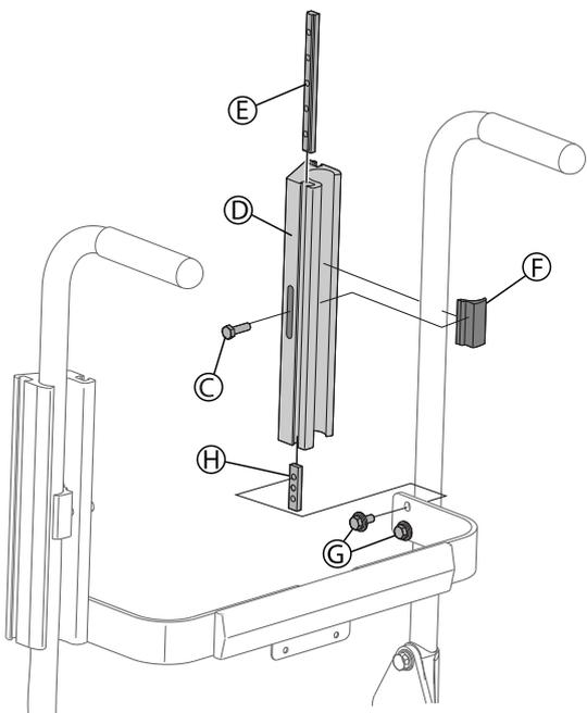
1. Remove hardware (C) securing the back mount (D) to the back canes.
