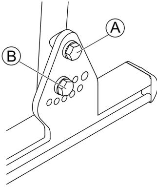
1. On both sides, loosen screw (A).
