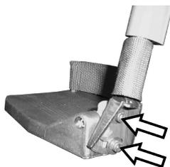
1. Use the Allen key to loosen both set screws on the foot plate.
