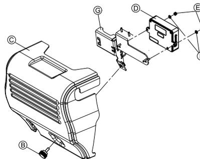
Fig. 15-6 Actuator Module Replacement—Powered Backrest
