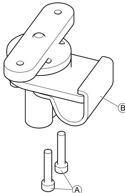
Loosen and remove screws (A) to unlock strap plate (B).
