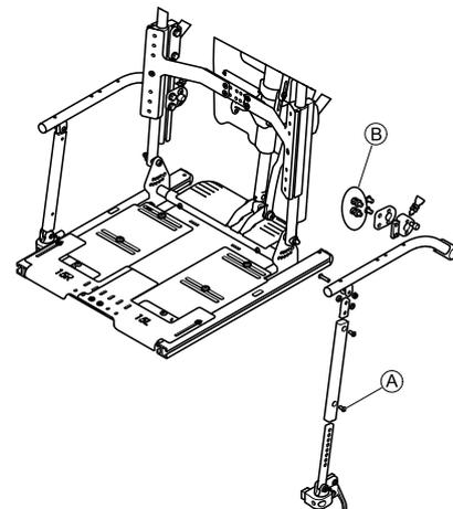
1. Remove screw **A** and slide the inner pivot arm up/down to the desired height.
