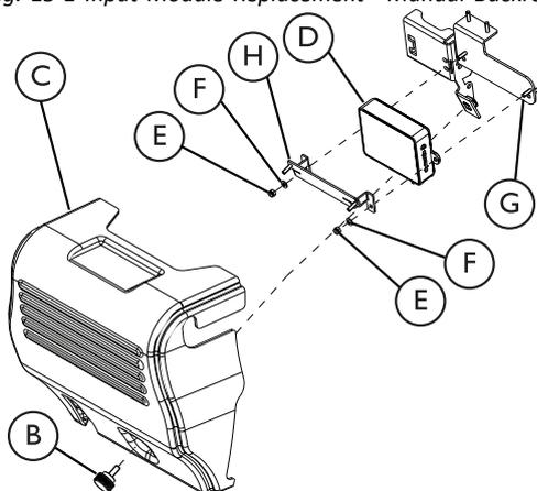
Fig. 15-2 Input Module Replacement—Powered Backrest
