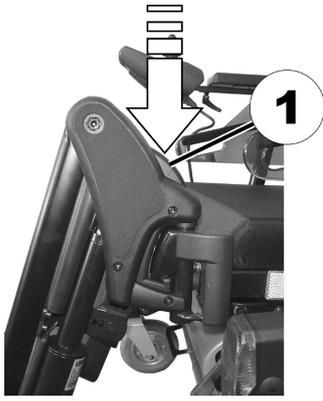
1. Press the unlocking button (1) and swivel the legrest outward.
